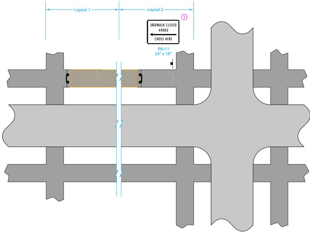
① Omit "SIDEWALK CLOSED AHEAD CROSS HERE" (R9-11) sign when closure is at sidewalk intersection as shown in layout 1.
