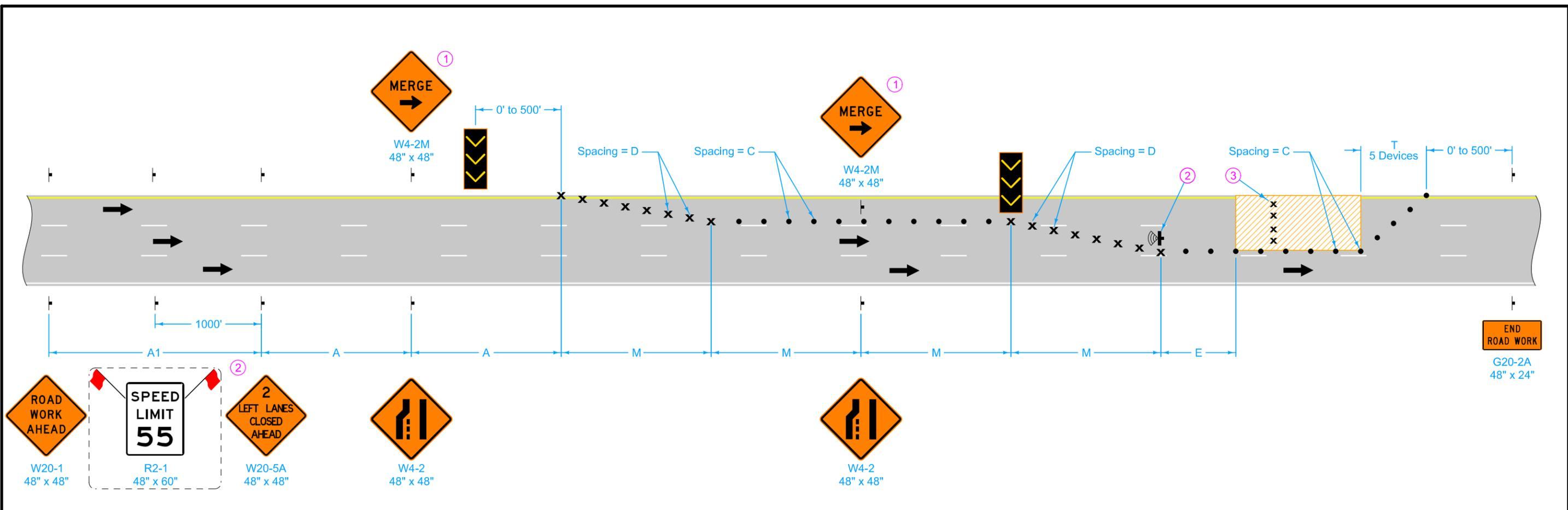
Where there is a lane line drop-off or rise, do not allow traffic to cross over the drop-off or rise, except for ramp locations where a BUMP (W8-1) sign is placed.
