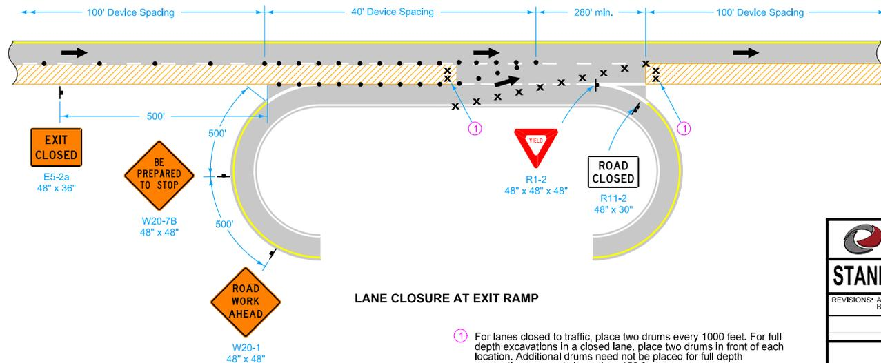
① For lanes closed to traffic, place two drums every 1000 feet. For full depth excavations in a closed lane, place two drums in front of each location. Additional drums need not be placed for full depth excavations spaced closer than 150 feet.
