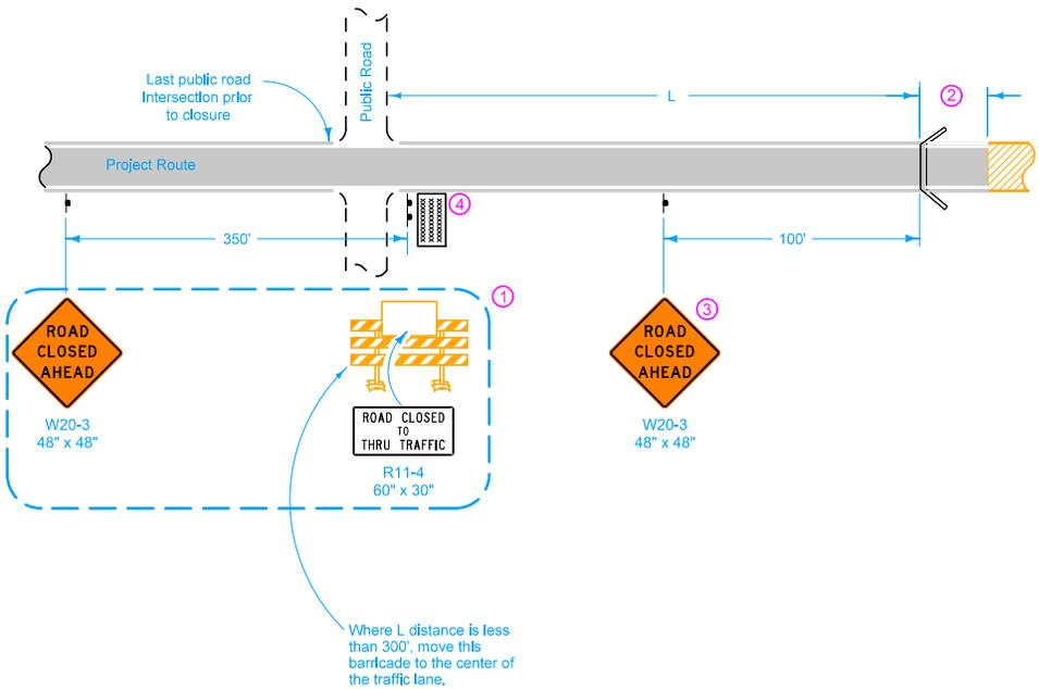
Where L distance is less than 300', move this barricade to the center of the traffic lane.
