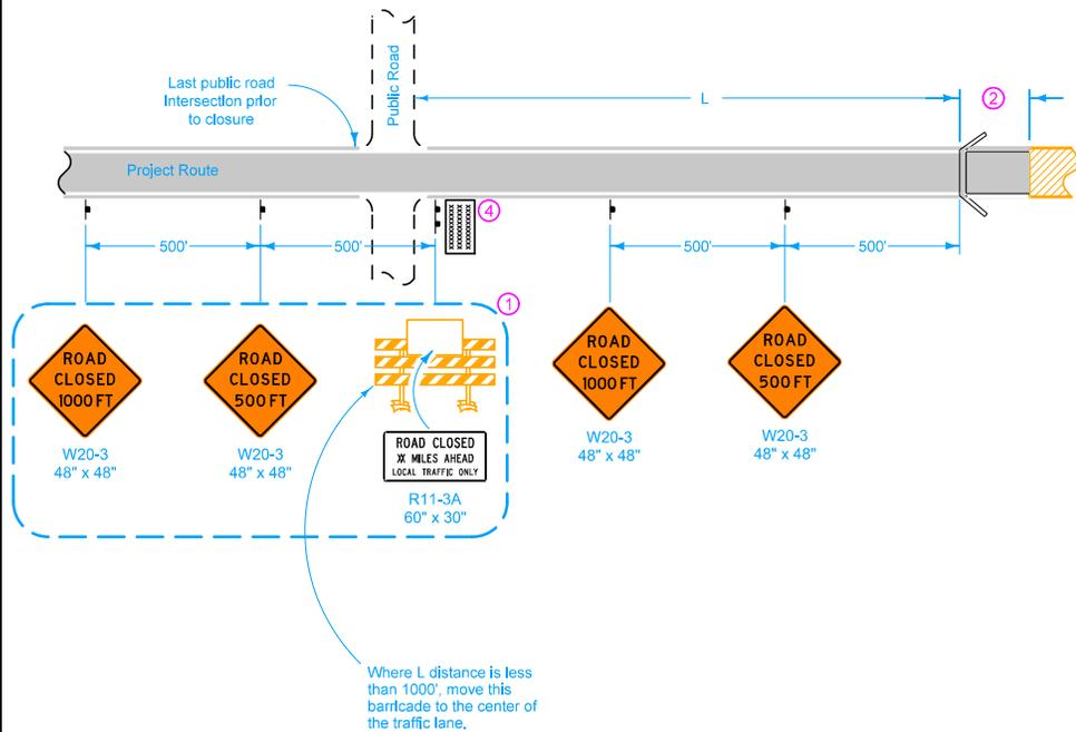
Where L distance is less than 1000', move this barricade to the center of the traffic lane.
