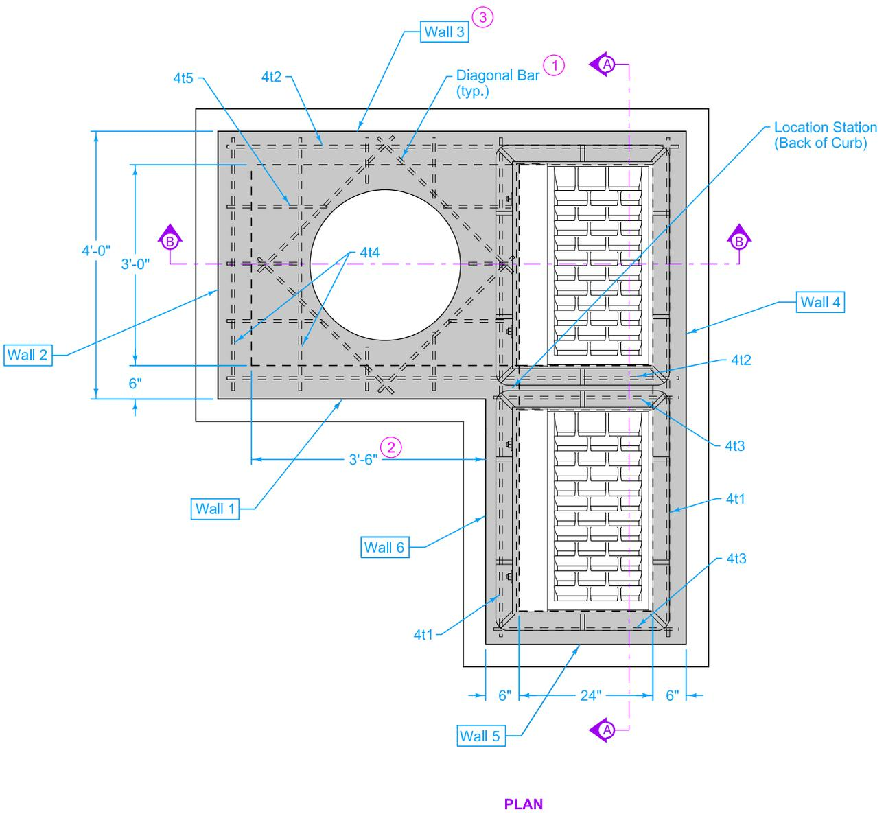
Maximum pipe diameters are set based on maximum structure depth of 6 feet-6 inches and the objective of placement of the centerline of the pipe on the centerline of the manhole opening for maintenance purposes.
