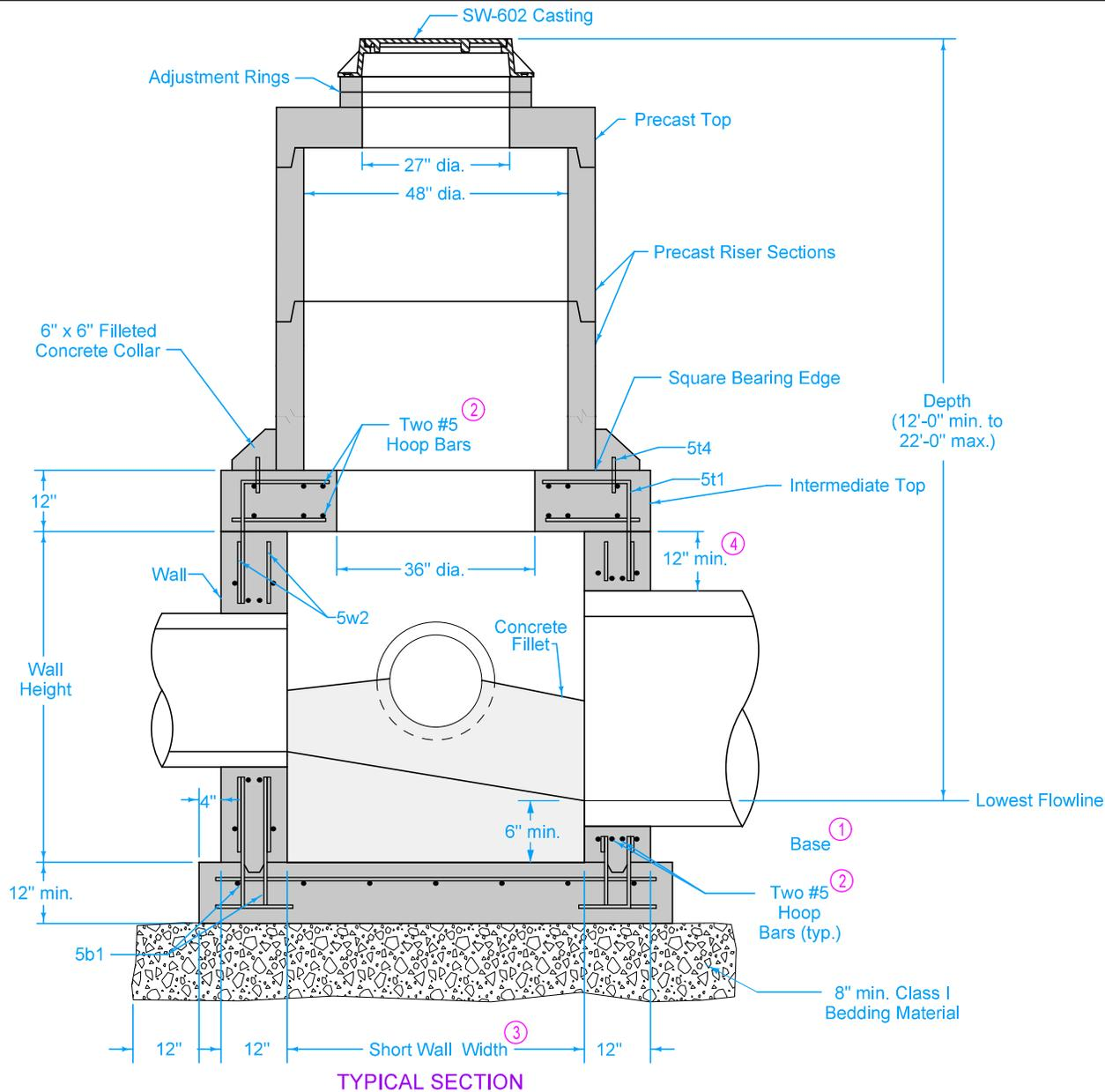
Adjacent walls may have different widths based upon pipe configuration, but structure must be rectangular.
