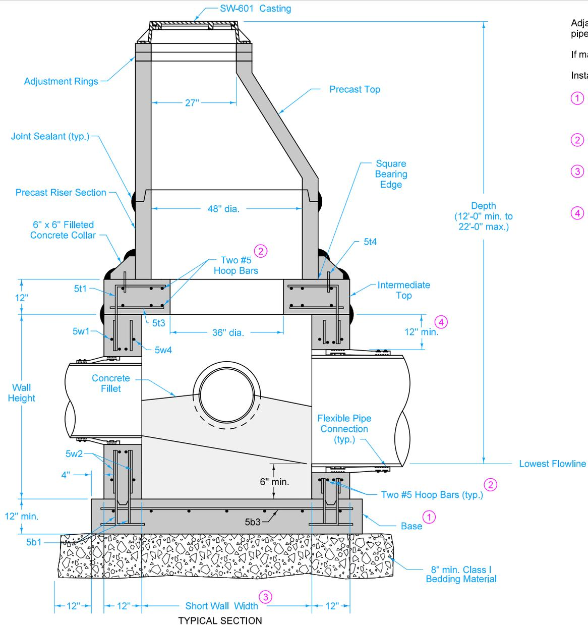
Adjacent walls may have different widths based upon pipe configuration, but structure must be rectangular.
