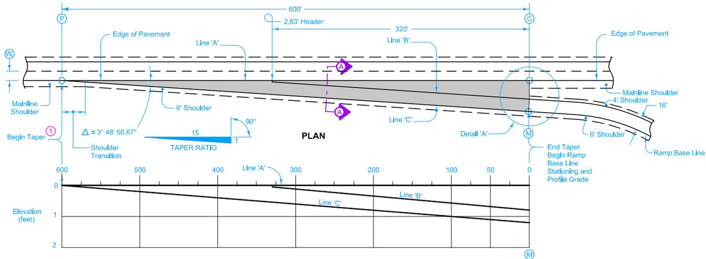
NOTE: The algebraic difference between profile grade for Ramp Base Line at (M) and relative profile grade of Mainline at (C) is 0.2%.
