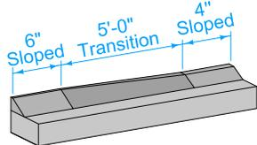
CURB TRANSITION FROM 6" SLOPED TO 4" SLOPED
