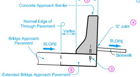
Install a 'C' joint in concrete approach barrier to match the location of each joint in both roadway and bridge approach pavement.
