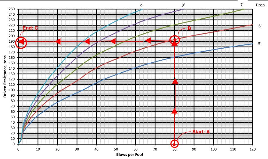
Start at point A, the Blows per foot you receive when driving, in this case it is 80 BPF. Follow up to your Ram rise, point B, this case it was a 6' Ram Rise End at point C, this is your end of drive driving resistance. In this case it is 190 Tons.
