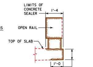
**CONCRETE SEALER LIMITS FOR OPEN RAILS**
