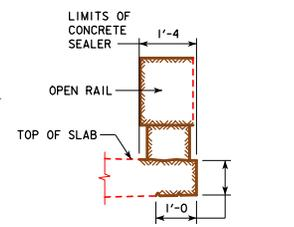
**CONCRETE SEALER LIMITS FOR OPEN RAILS**
