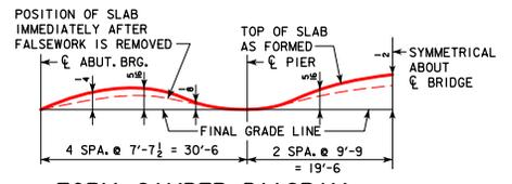
THIS DIAGRAM SHOWS THE FORM CAMBER REQUIRED TO COMPENSATE FOR THE ANTICIPATED ULTIMATE DEAD LOAD DEFLECTION. THE ABOVE DIMENSIONS DO NOT INCLUDE ANY ALLOWANCE FOR FORM DEFLECTION OR FALSEWORK SETTLEMENT.
