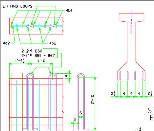
2 TOP DEFLECTED OR STRAIGHT STRANDS ARE TO BE CUT WITH 1'-0" PROJECTIONS AND SHOP BENT UP OR DOWN AS SHOWN (BEND TOP AND BOTTOM ROWS). THE REMAINING TOP STRANDS ARE TO BE CUT WITH 0'-3" PROJECTIONS. FOUR BOTTOM STRANDS ARE TO BE CUT WITH 1'-0" PROJECTIONS AND SHOP BENT AS SHOWN. THE REMAINING BOTTOM STRANDS SHALL BE CUT OFF REASONABLY FLUSH WITH THE CONCRETE.
