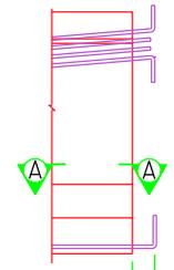
**STRAND PROJECTION AT BEAM ENDS WHEN EMBEDDED IN CONCRETE END DIAPHRAGMS**
