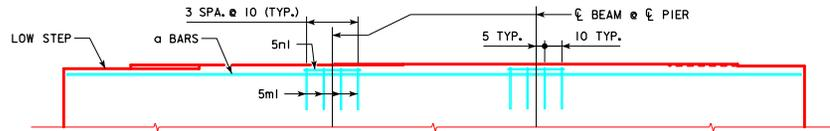
**PART ELEVATION VIEW OF PIER CAP**
