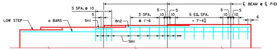
**PART ELEVATION VIEW OF PIER CAP**
