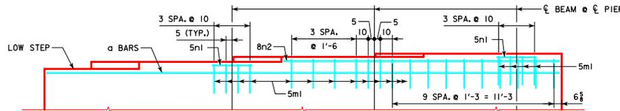
**PART ELEVATION VIEW OF PIER CAP**
