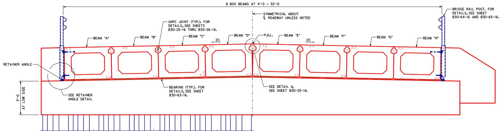
SECTION NEAR ABUTMENT WITH SHEET PILE WINGS
