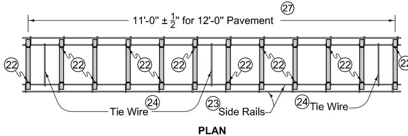
Spaces between dowel bars are nominal dimensions with a  $\frac{1}{4}$ " allowable tolerance.
