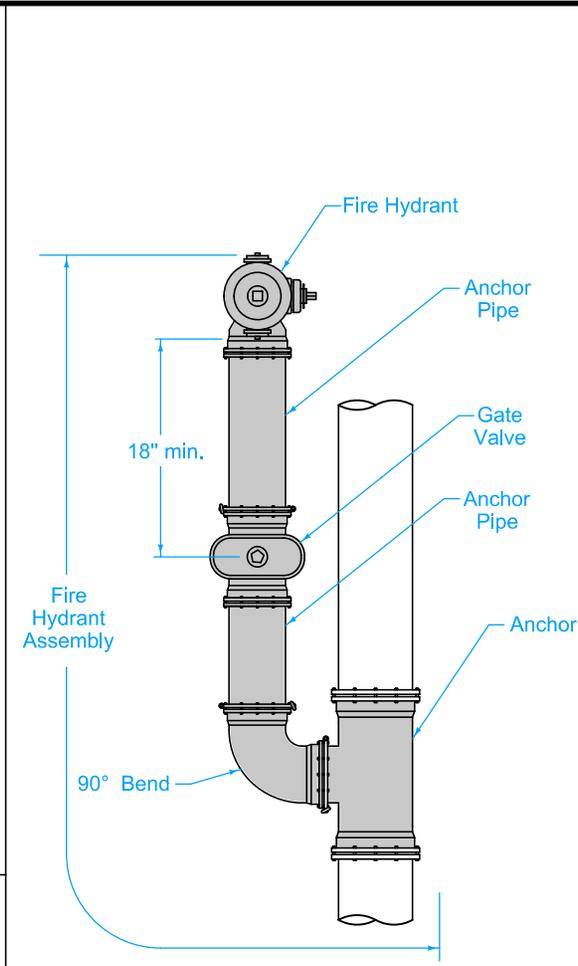
Use ductile iron pipe with restrained mechanical joints for fire hydrant assembly and anchor tee.
