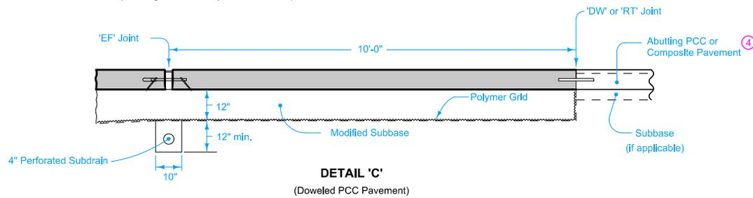
④ If abutting pavement (PCC or HMA) is not in place, refer to BR-213.
