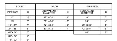
Provide guard dimensions to fit with type of apron provided. Ensure 'V' Bar completely rests on apron.
