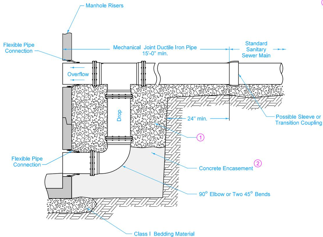
Construct drop and overflow from ductile iron pipe of same diameter specified for sewer main. Provide mechanical joints for all ductile iron pipe and fittings.
