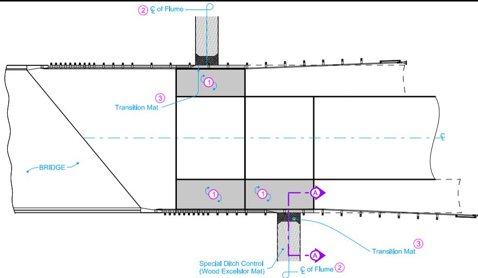
Price bid for "Bridge End Drain, DR-401" is full compensation for furnishing, installing, and constructing the Bridge End Drain as shown.
