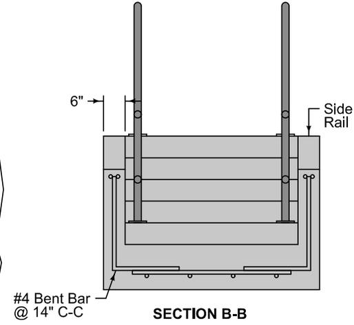
Provide a minimum of 2 inches of cover for all reinforcing.
