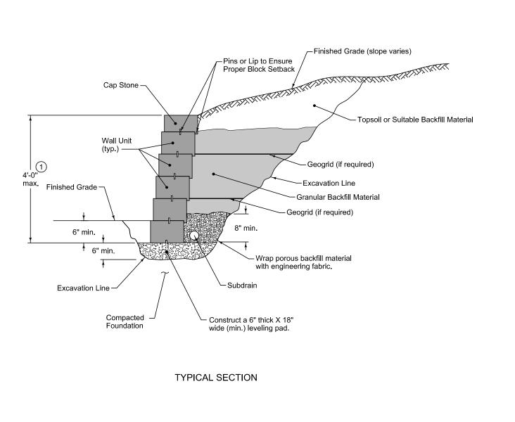
Exact dimensions, wall batter, backfill limits, reinforcement, and leveling pad materials and dimensions will be specified by the wall manufacturer.
