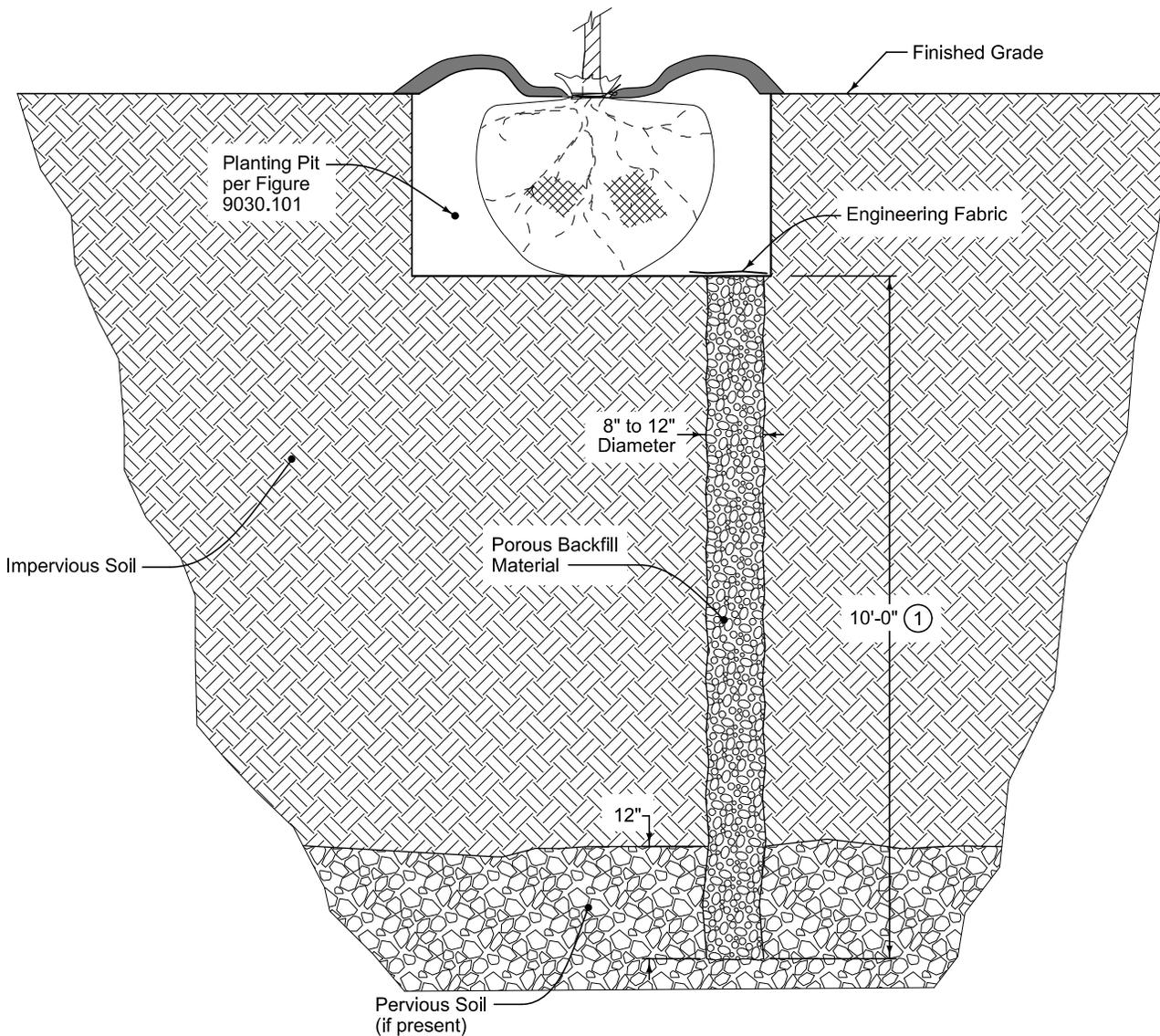
① If pervious soil is encountered at a depth less than 10 feet, the drainage well may be terminated when the well extends a minimum of 12 inches into the pervious soil layer.
