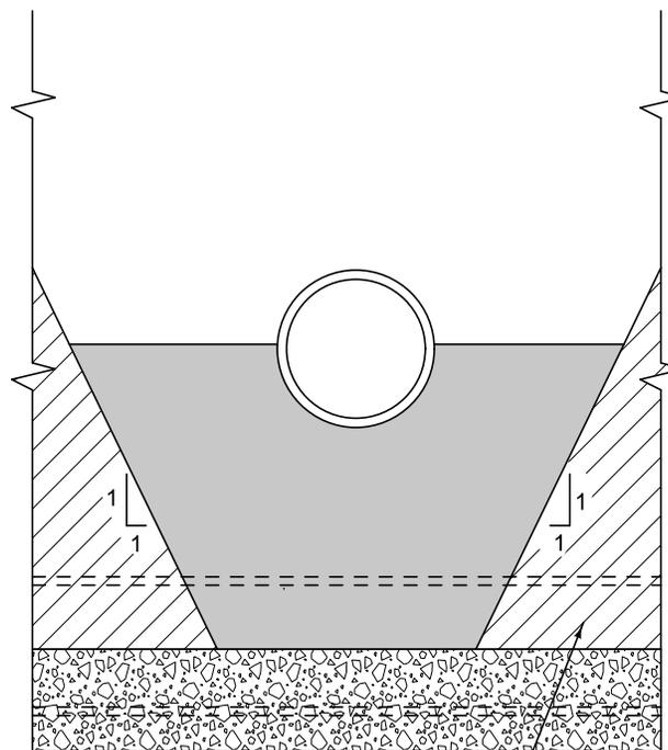
Use flowable mortar utility line support when new utility excavation is crossing under an existing utility line (sewer lines, water lines, gas lines, etc.) as directed by the Engineer.
