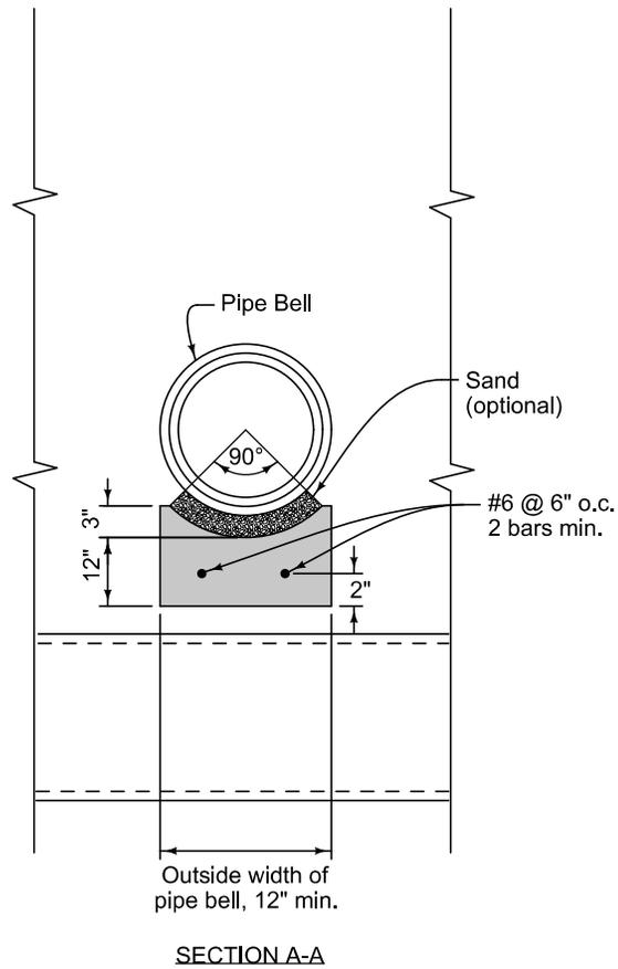
Use reinforced concrete beam utility line support when new sewer excavation is crossing under an existing utility line (sewer lines, water lines, gas lines, etc.) as directed by the Engineer.
