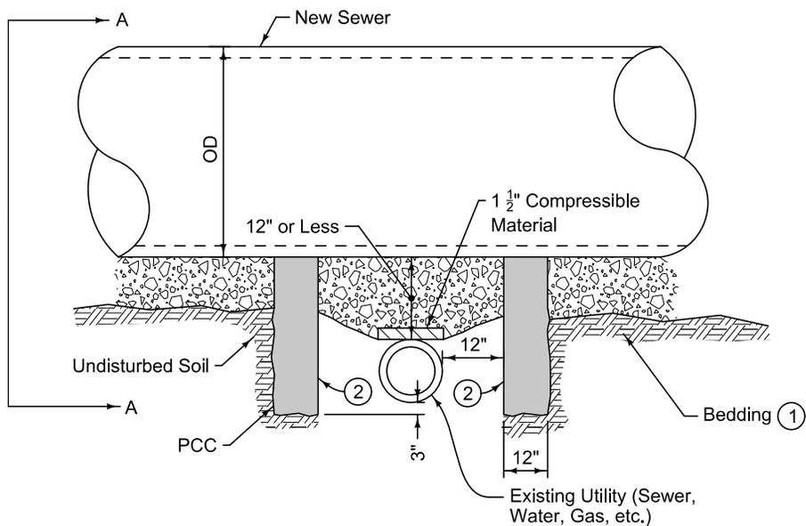
Install pipe support for all new sewers 12 inches in diameter or larger when clearance between bottom of new sewer and top of existing line is 12 inches or less.
