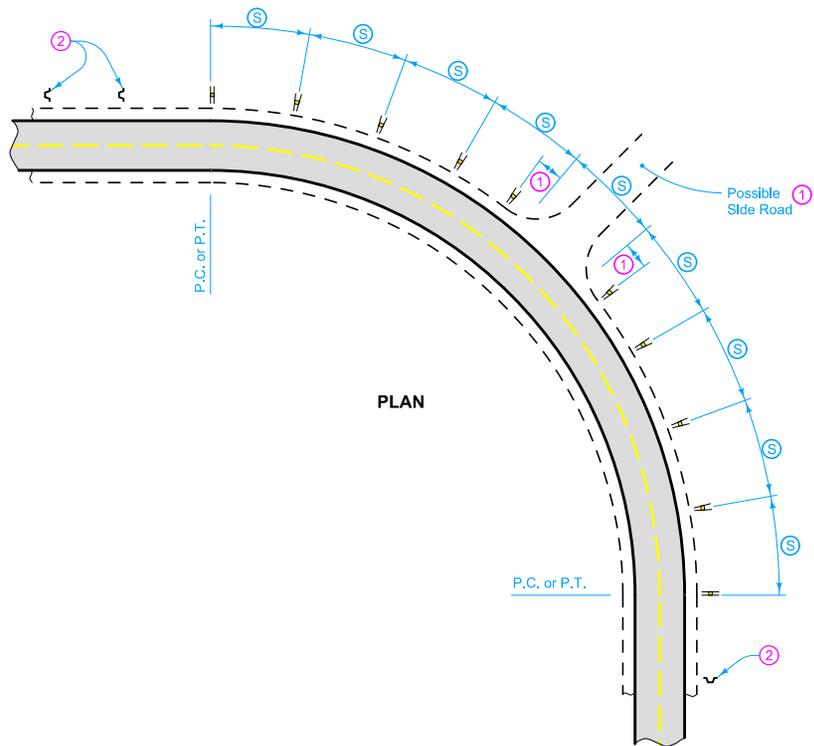
To be effective, Chevron Sign Panels should be visible for at least 500 feet. Attach Chevron Sign Panels to the adjustable brackets at an angle so headlight beams are not reflected back into the driver's eye.
