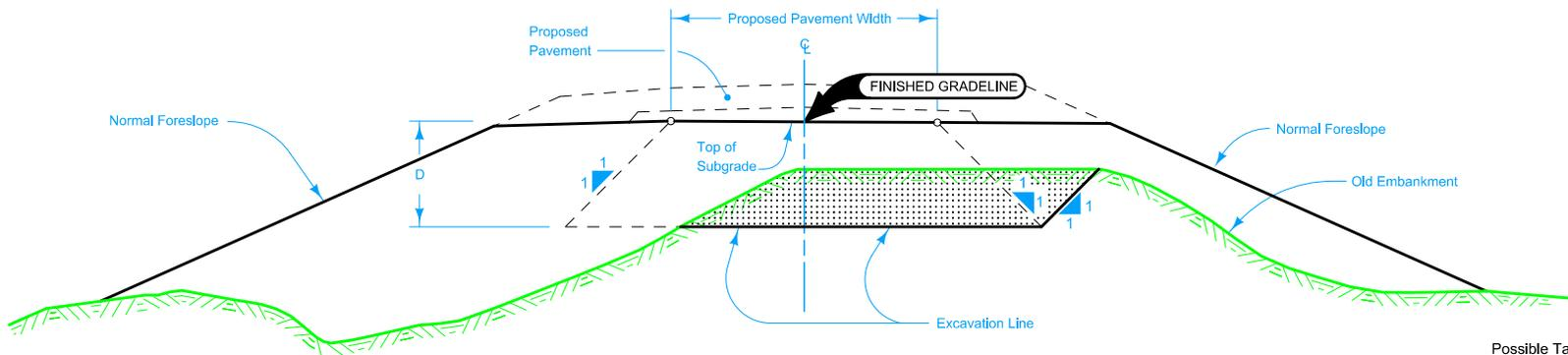
TYPICAL CROSS SECTION REBUILDING EMBANKMENT
