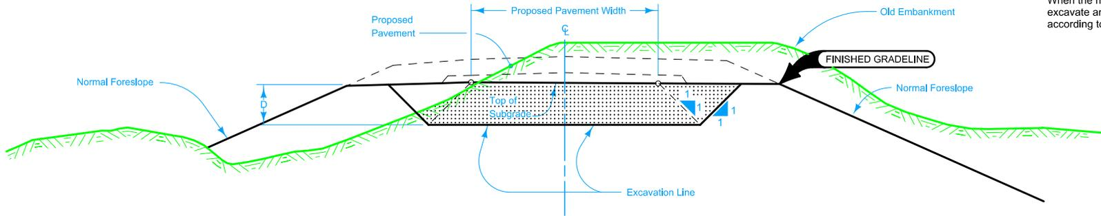
TYPICAL CROSS SECTION REBUILDING EMBANKMENT
