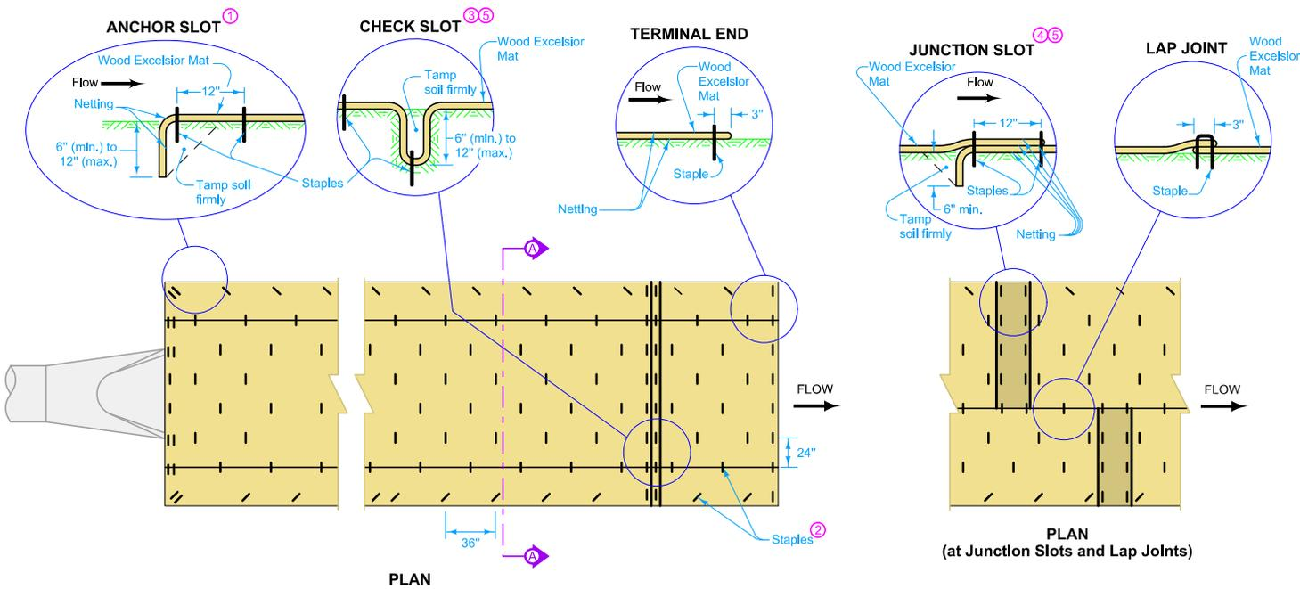
Provide necessary excavation at locations where silt conditions require shaping of a ditch to provide a proper type of area for installation of wood excelsior mat for special ditch control.
