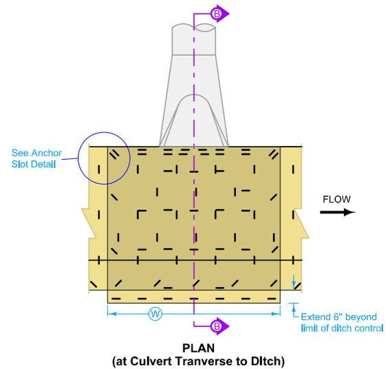
PLAN (at Culvert Transverse to Ditch)
