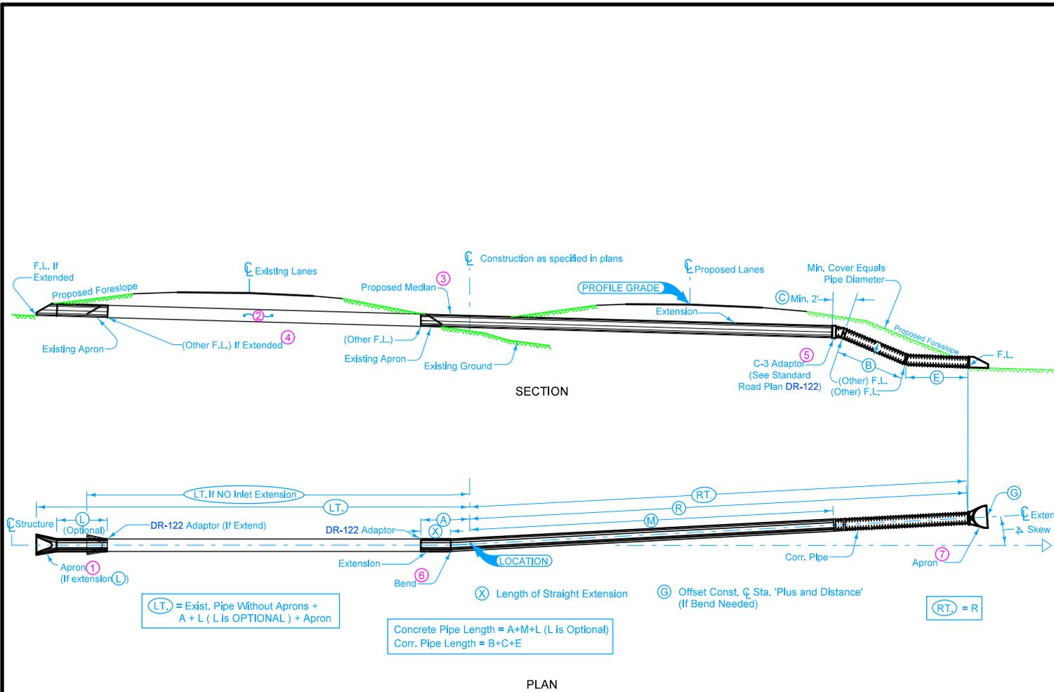
If bend is required, extend in the direction specified with skew measured from centerline of existing structure. Dimension Rt. or Lt. is measured at  $\phi$  of pipe along laying length.
