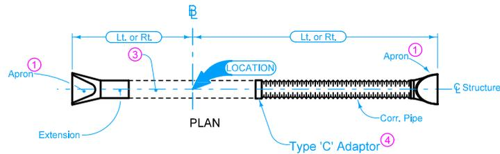
$\bar{E}$  is  $\bar{C}$  of roadway, dike, survey, or other as detailed on plans.
