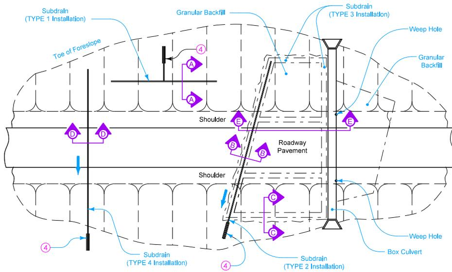
PLAN VIEW OF TYPICAL STANDARD SUBDRAIN INSTALLATIONS
