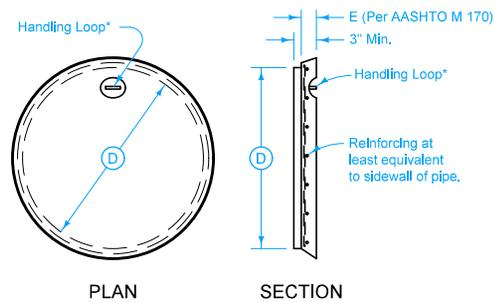
\*The handling loop may be omitted when the cap is placed in a buried installation.
