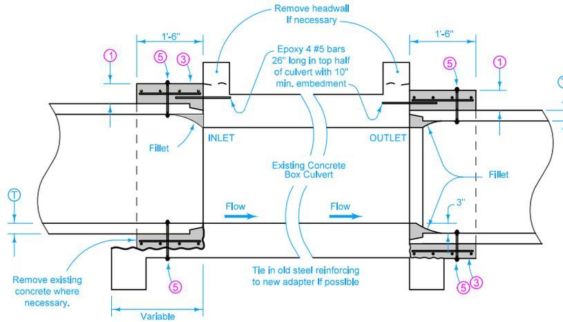
CONCRETE PIPE TO CONCRETE BOX CULVERT
