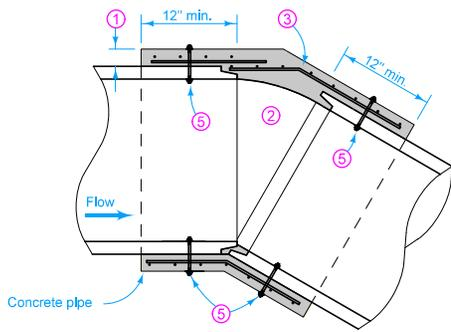
CONCRETE PIPE TO CONCRETE PIPE
