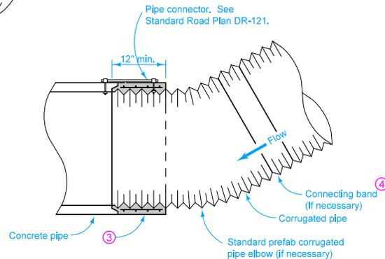
CORRUGATED PIPE TO CONCRETE PIPE
