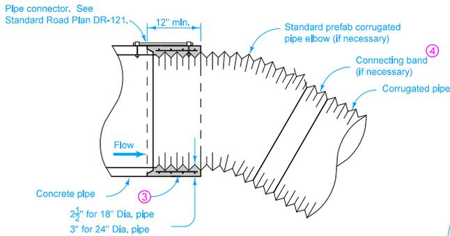
CONCRETE PIPE TO CORRUGATED PIPE
