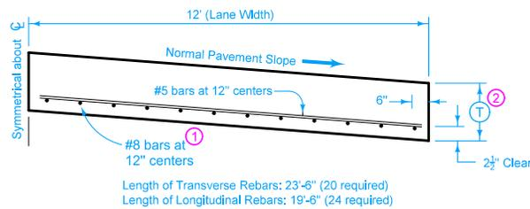
Use the same concrete for the bridge approach section as is used for the remainder of the project pavement.
