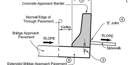
Install a 'C' joint in concrete approach barrier to match the location of each joint in both roadway and bridge approach pavement.
