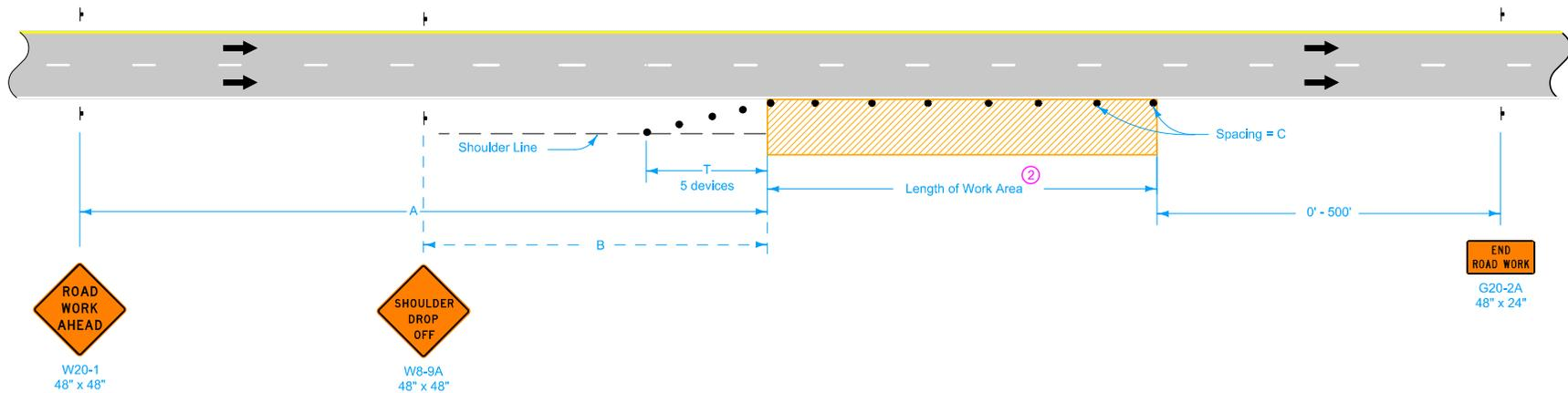
When a pavement edge drop-off exists, install a SHOULDER DROP-OFF sign.
