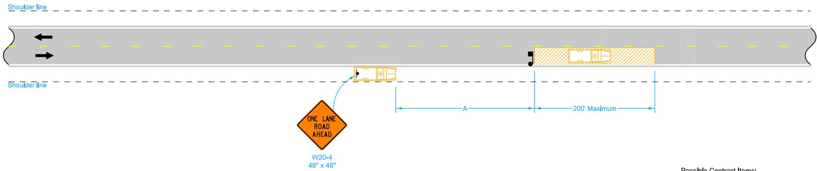
This layout is intended for use with slow-moving operations or with operations involving stops not to exceed 15 minutes. For stops exceeding 15 minutes or in heavy traffic situations, use TC-213.
