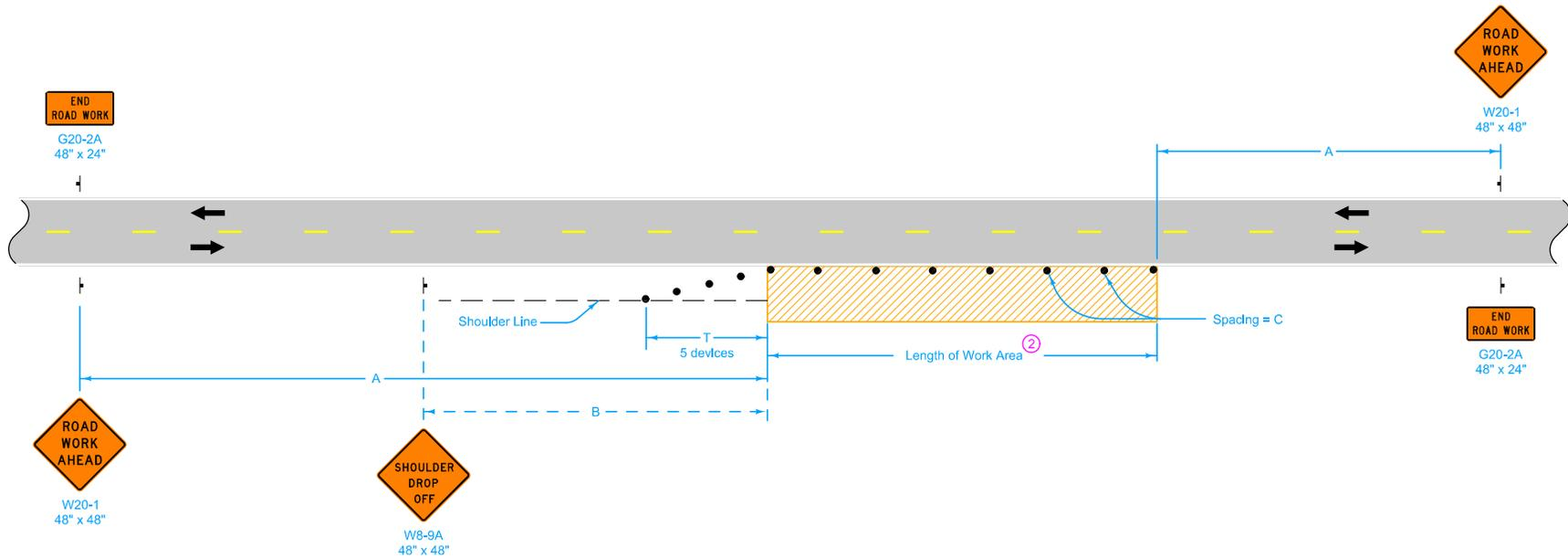
When a pavement edge drop-off exists, install a SHOULDER DROP-OFF sign.
