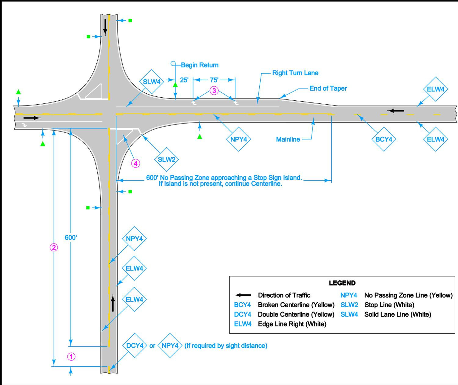
Roadways may or may not have edge lines. When the free flow roadway has edge lines but the stop controlled roadway does not, end edge lines at the end of returns (marked by ▲s). When the stop controlled roadway has edge lines but the free flow roadway does not, end edge lines at the end of returns (marked by ■s). If both roadways have edge lines, continue edge lines around the returns.
