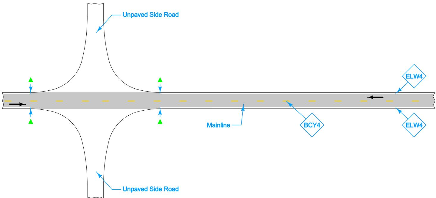
Roadways may or may not have edge lines. When the free flow roadway has edge lines but the stop controlled roadway does not, end edge lines at the end of returns (marked by ▲s). When the stop controlled roadway has edge lines but the free flow roadway does not, end edge lines at the end of returns (marked by ■s). If both roadways have edge lines, continue edge lines around the returns.
