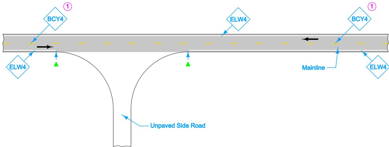
Roadways may or may not have edge lines. When the free flow roadway has edge lines but the stop controlled roadway does not, end edge lines at the end of returns (marked by ▲s). When the stop controlled roadway has edge lines but the free flow roadway does not, end edge lines at the end of returns (marked by ■s). If both roadways have edge lines, continue edge lines around the returns.
