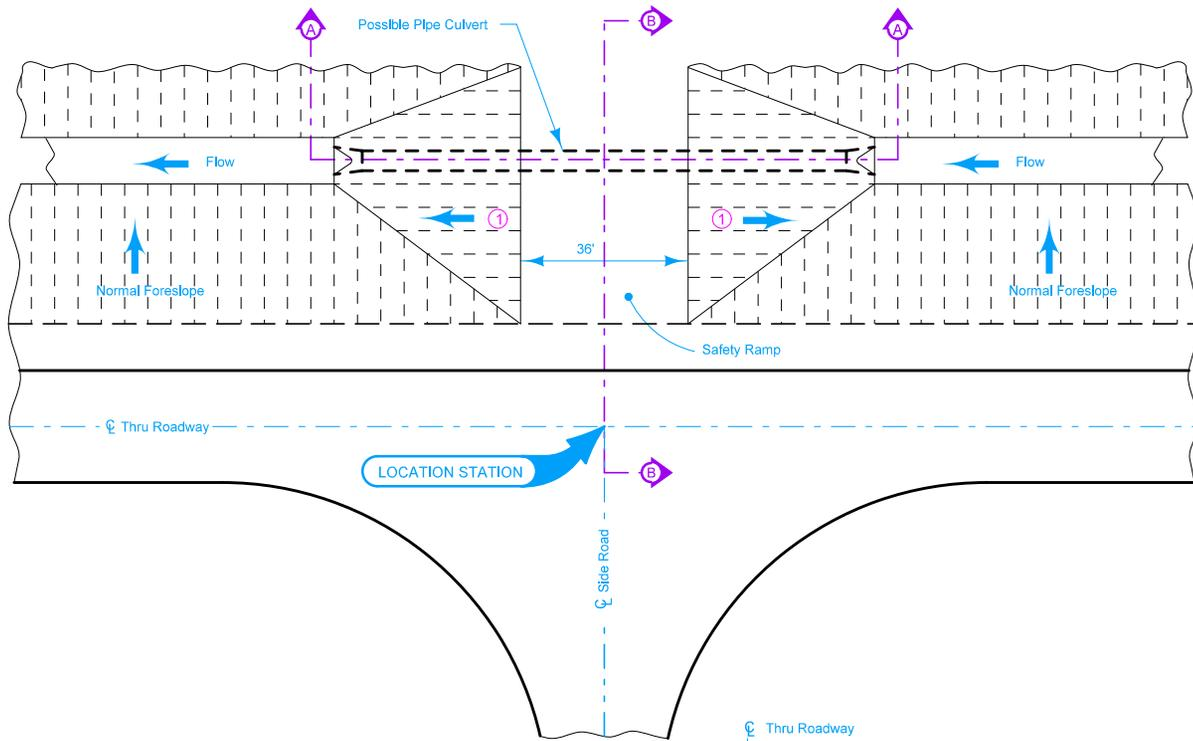
① Slope 10:1 or flatter without pipe, 8:1 or flatter with pipe.
