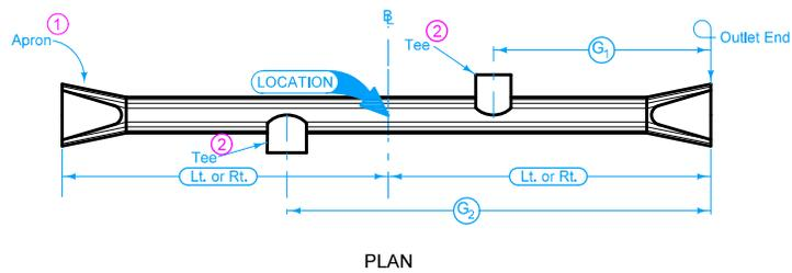
REINFORCED CONCRETE PIPE CULVERT
