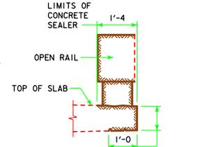
**CONCRETE SEALER LIMITS FOR OPEN RAILS**
