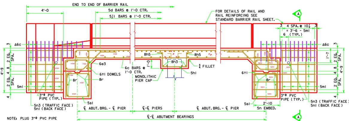
NOTE: PLUG 3" PVC PIPE WITH EXPANDING FOAM PRIOR TO BACKFILLING BEHIND ABUTMENTS.
