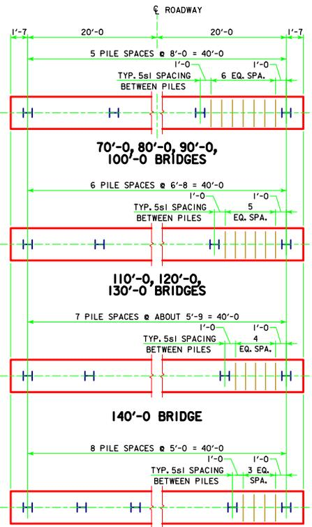
**PILE PLAN - 0° SKEW STEEL PILING**
